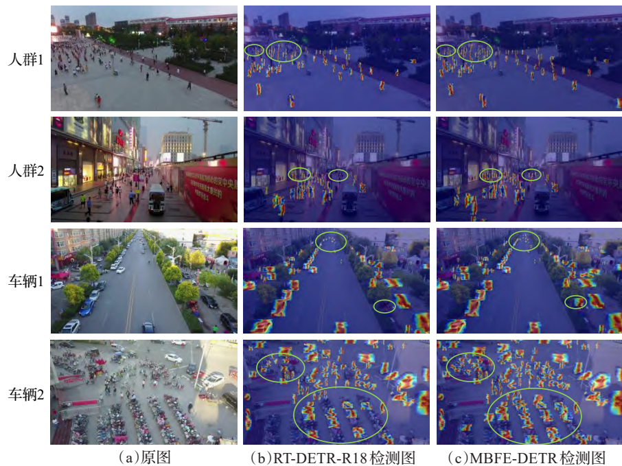
图8 MBFE-DETR 和RT-DETR-R18 的热力图对比 Fig.8 Comparison of heat maps between MBFE-DETR and RT-DETR-R18
